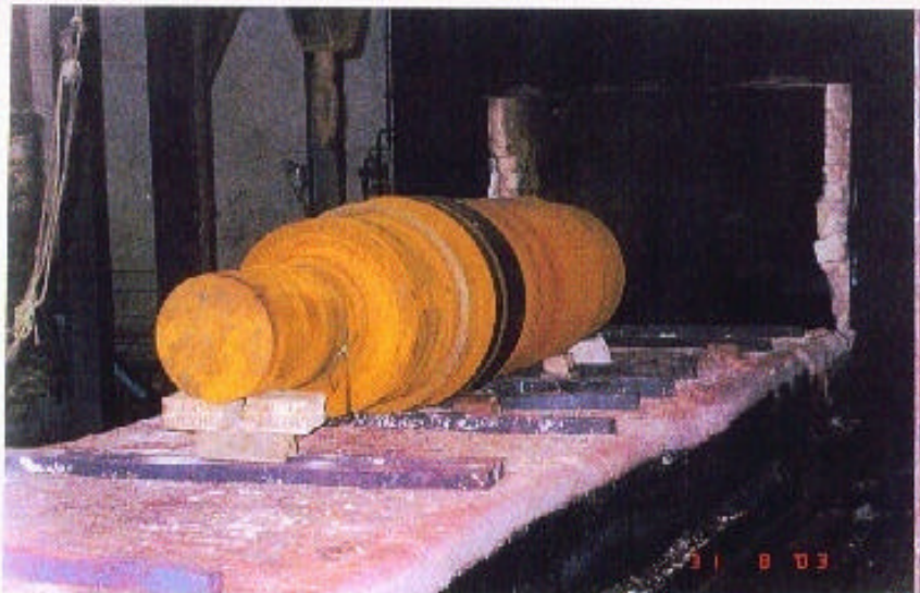
Proof Machined Stepped Shaft being loaded into Furnace for Stress Relieving.
