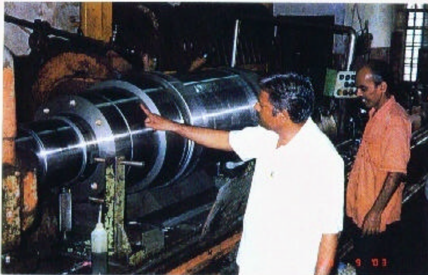
Shri Kishan Singh Ji of M/s. Lakshmi Cement checking fully ground shaft. Grinding carried out on 6 mtrs. center to center grinding m/c.
