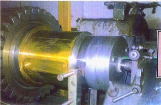
Golden Antirust being applied on the ground area to prevent oxidation.
