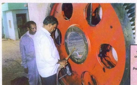
Team of two welders continuously stationed to weld bore.
