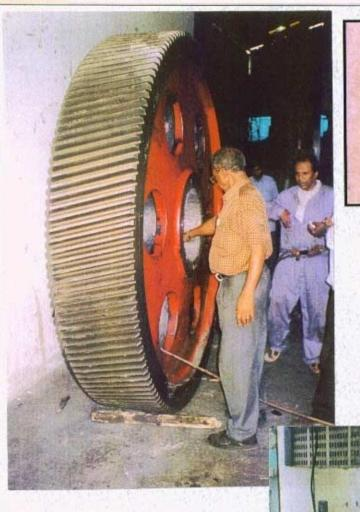
Gear BORE being Inspected for welding splatter, correctness of welding and uniformity of lay by our Inspector.
