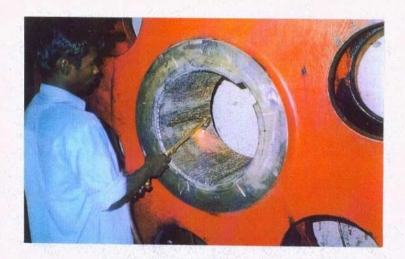
Post Heating of the bore to be carried out so as to keep the temperature uniform and prevent cracking of the welded area.
