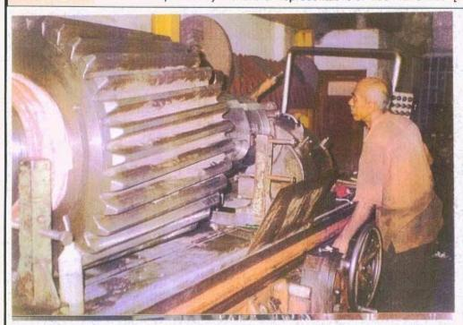
Final Shaft diameter being ground to size using bluing paste.
