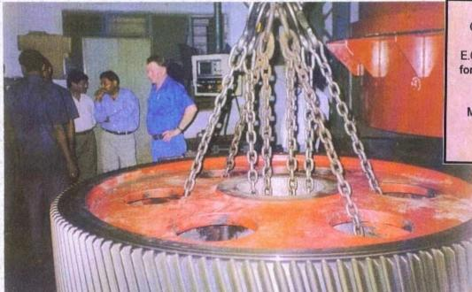
Gear Wheel is being transported by E.O.T (30 T) to the V.T.L. for taking up machining of Bore.
