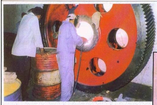
Welding continues as build up of metal increases layer by layer.
