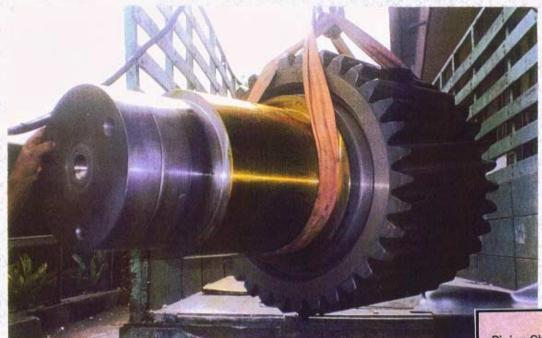
Pinion Shaft is supported on wooden supports and bearing and ground areas are packed with rubber sheet to prevent damage in transit. [Rope tied to secure pinion.]
