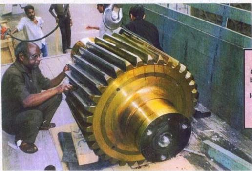
Golden Antirust Lacquer being applied over entire surface of Pinion post loading it into the vehicle prior to dispatch.
