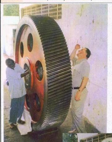
F.L.Smidth's representative checking gear and seeing if any rectification of welding is required.
