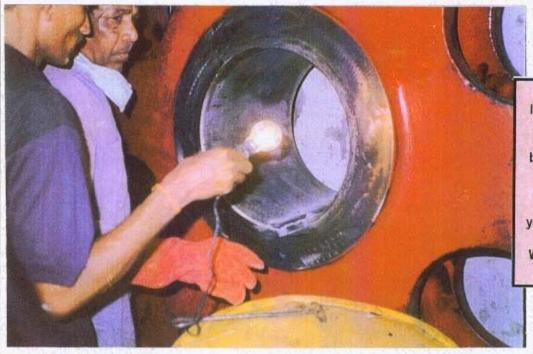
Inspection of Gear Bore after welded run to ensure uniformity of bead and proper fusion.
