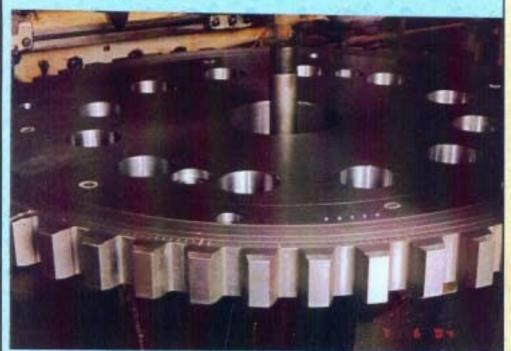
CLOSE UP OF TURNING GEAR WITH SERRATIONS AND FULLY MACHINED HOLES.
