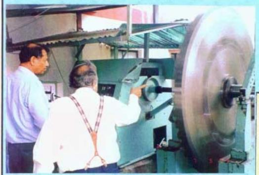
FULLY DYNAMICALLY BALANCED JOB ROTATING AT 375 RPM
