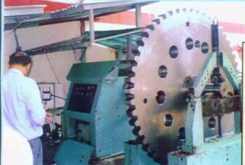
FULLY RE-MACHINED GEAR LOADED ON DYNAMIC BALANCING MACHINE
