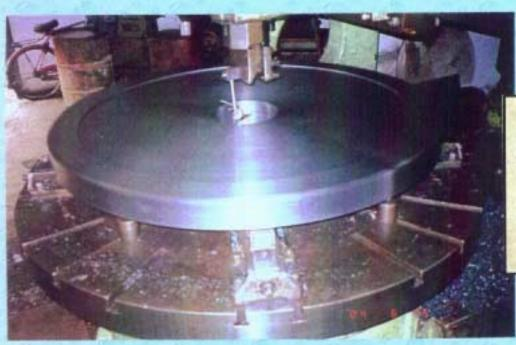
FULL MACHININIG OF ONE FACE AND BORE OF GEAR BLANK COMPLTED.
