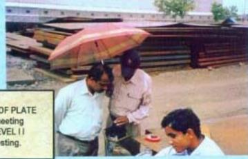
100 % SCANNING OF PLATE BEING DONE meeting ASTM A 578 LEVEL II Standard of Testing.
