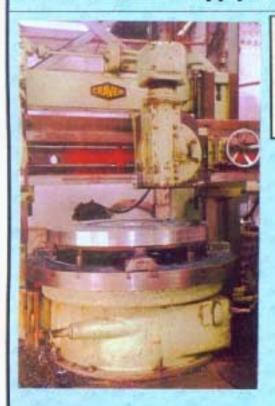
IMPORTED CRAVEN VERTICAL TURRET LATHE[V.T.L] being used for machining gear blank. High speed and feed cut being taken seeing urgency of Job.
